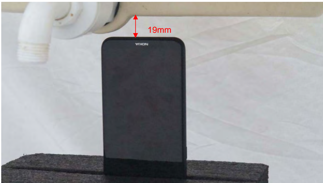
Picture 20: Front Side, the distance from handset to the bottom of the Phantom is 19mm
