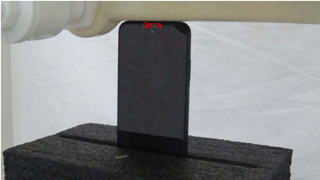
Picture 17: Top Side, the distance from handset to the bottom of the Phantom is 0mm
