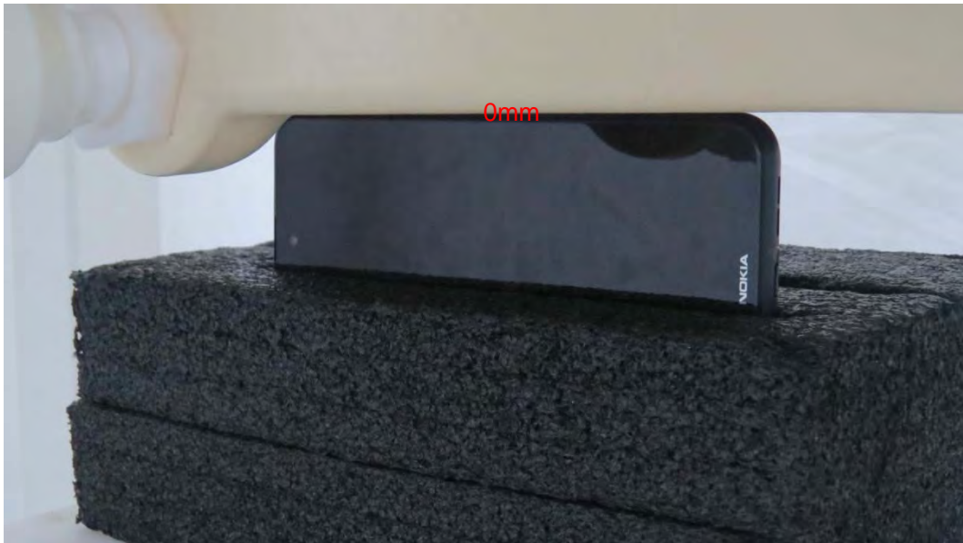
Picture 16: Right Side, the distance from handset to the bottom of the Phantom is 0mm
