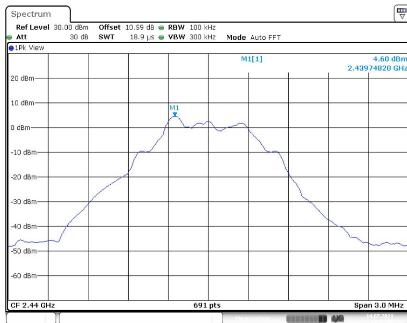
Fig.54 Conducted Spurious Emission (CH19, Center Frequency), LE Coded S=8
