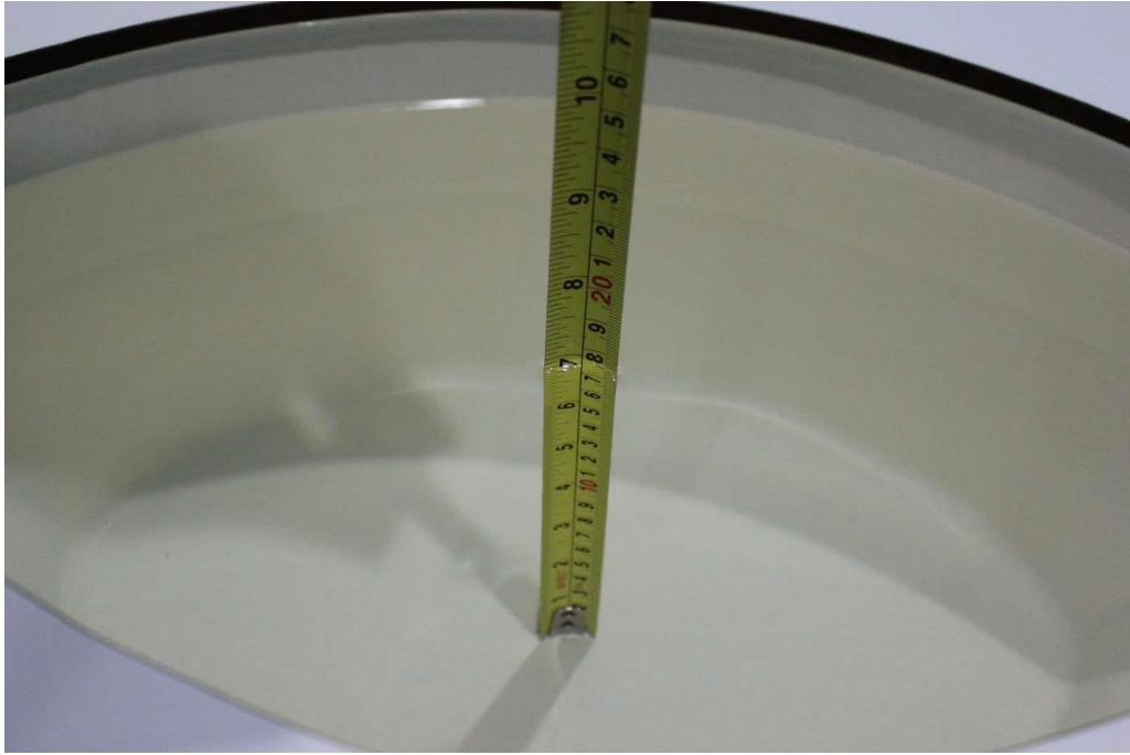
Picture 7-7: Liquid depth in the Flat Phantom(5GHz)
