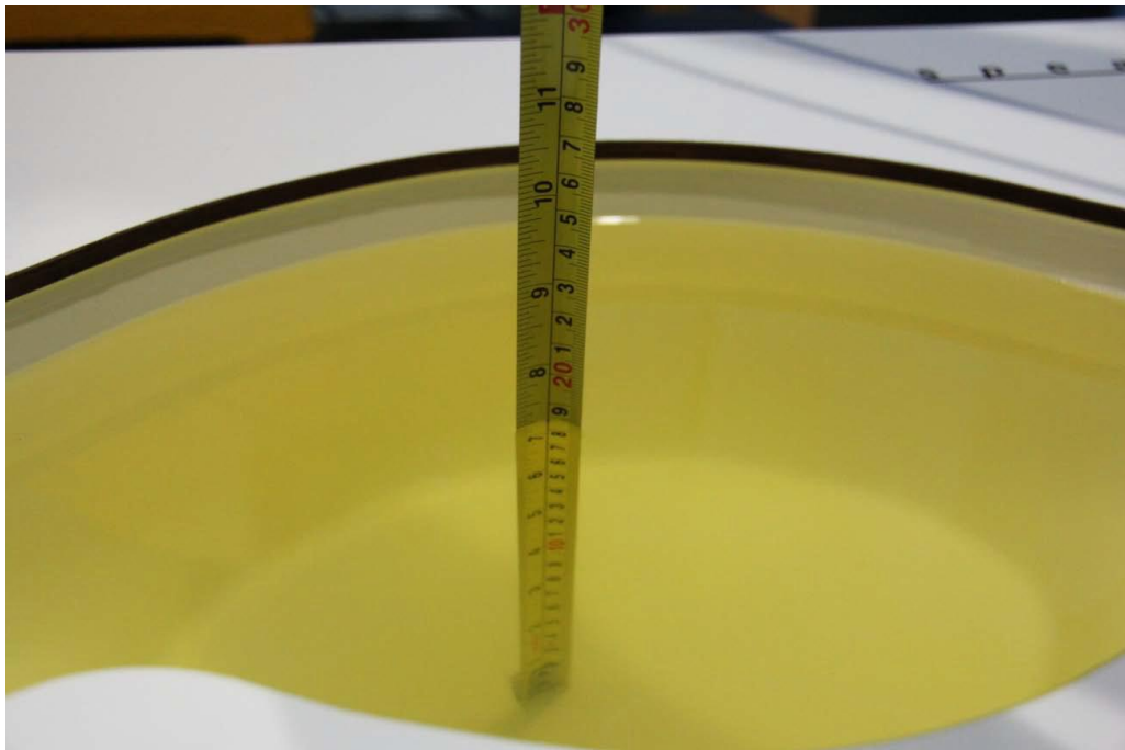
Picture 7-5: Liquid depth in the Flat Phantom(2450MHz)
