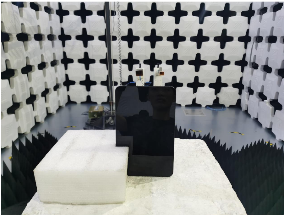
16. Radiated Emissions (Part 15C, 18GHz -26.5GHz)
