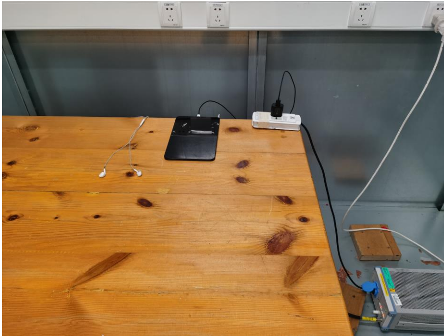
21. Conducted Emission (Part 15B, FM receiver)
