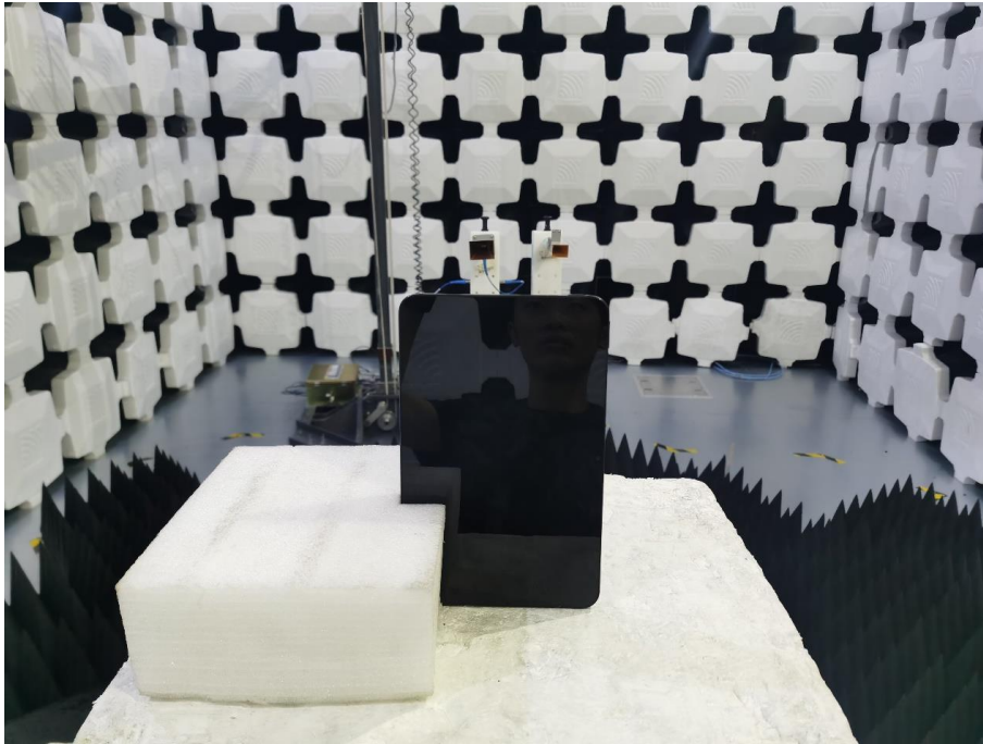
19. Radiated Emissions (Part 22/24/27, 18GHz -26.5GHz)
