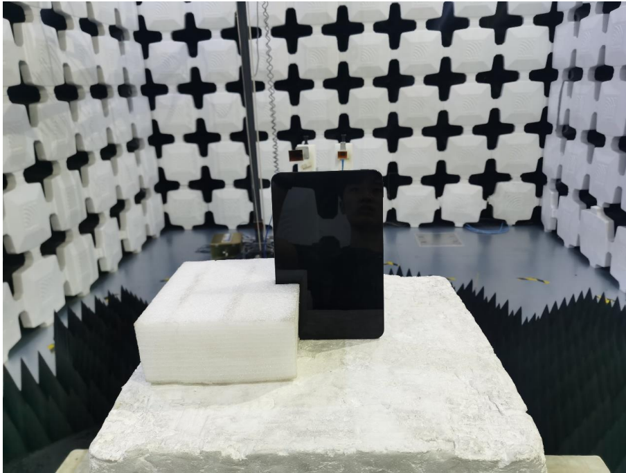
17. Radiated Emissions (Part 15C, 26.5GHz -40GHz)
