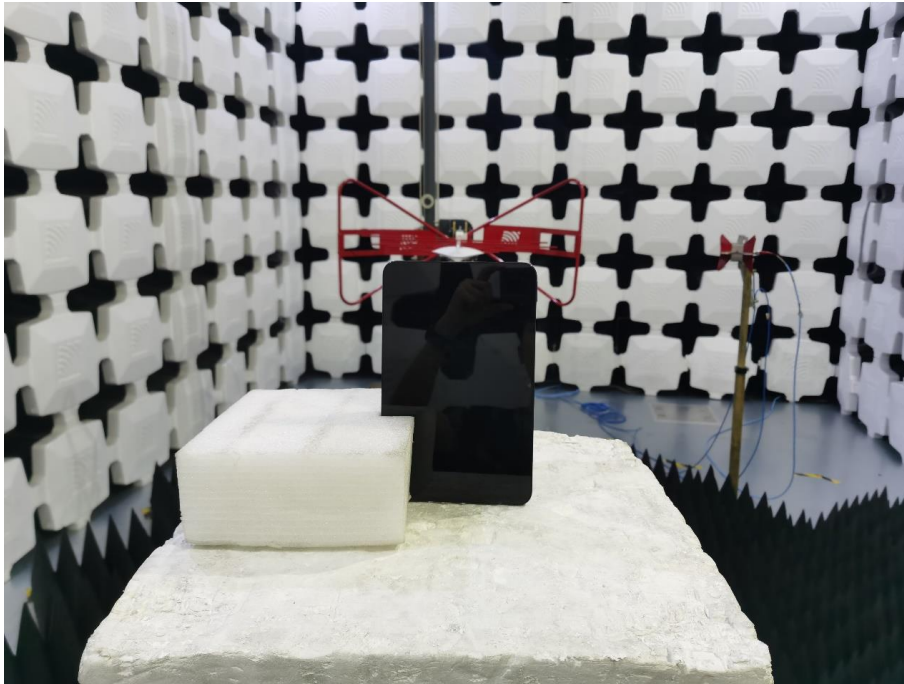
15. Radiated Emissions (Part 15C, 1GHz -18GHz)
