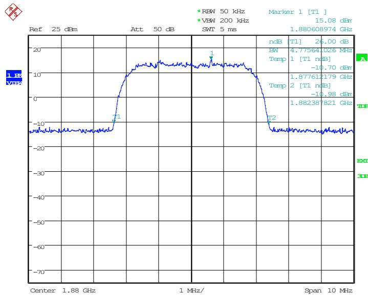
**Channel 9538-Emission Bandwidth (-26dBc BW)-QPSK**
