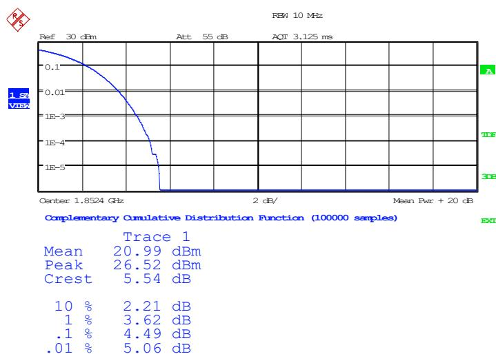
**Channel 9400- Peak-To-Average Power Ratio(PAPR)-QPSK**
