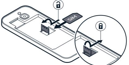
4. If you have a dual-SIM phone, slide the SIM2 holder to the right and open it up. Place the nano-SIM in the SIM2 slot face down, close down the holder and slide it to the left to lock it in place. Both SIM cards are available at the same time when the device is not being
