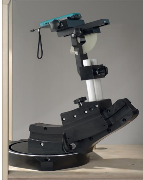
F-2. Device Holder for Transmitters
