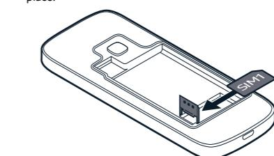
4. If you have a dual-SIM phone, slide the SIM card holder of the SIM2 slot to the right and open it up. Place the nano-SIM in the SIM2 slot face down, close down the holder, and slide it to the left to lock it in place. Both
