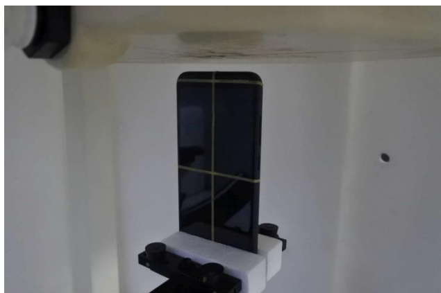
Top side, Test Separation 10 mm
