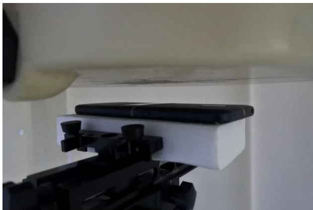
Back, Test Separation 19 mm
