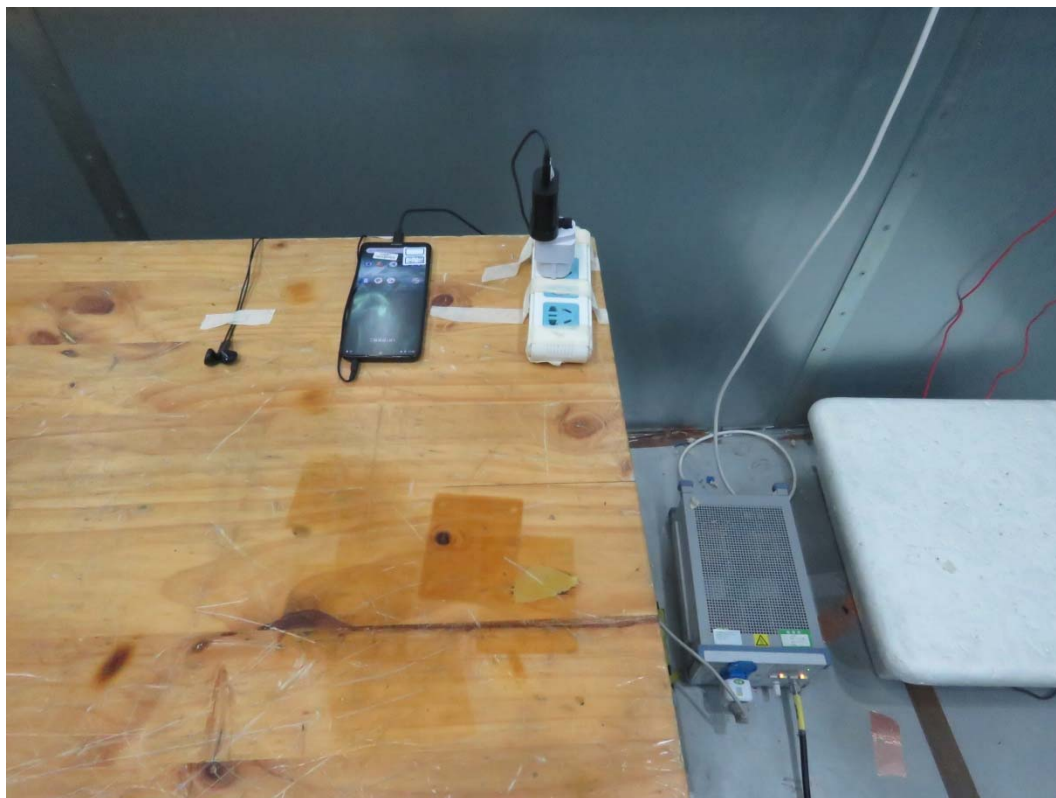
Picture 2 Conducted Emission Test Setup
