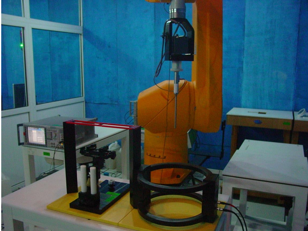
Picture A1: HAC T-Coil System Layout
