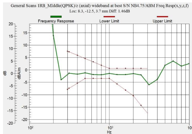
Figure C.14 Frequency Response of LTE B2 - OTT VoIP
