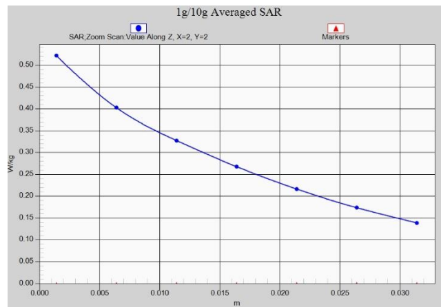
Fig. 1-1 Z-Scan at power reference point (GSM850)
