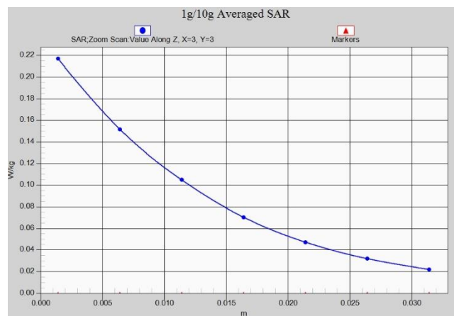
Fig. 1-7 Z-Scan at power reference point (WCDMA1700)
