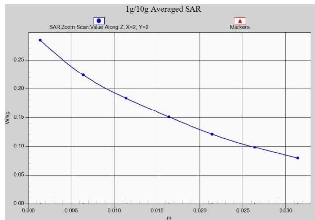
Fig. 1-9 Z-Scan at power reference point (WCDMA850)
