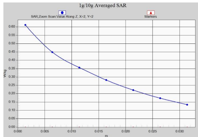
Fig. 1-10 Z-Scan at power reference point (WCDMA850)
