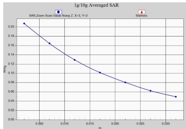
Fig. 1-1 Z-Scan at power reference point (GSM850)
