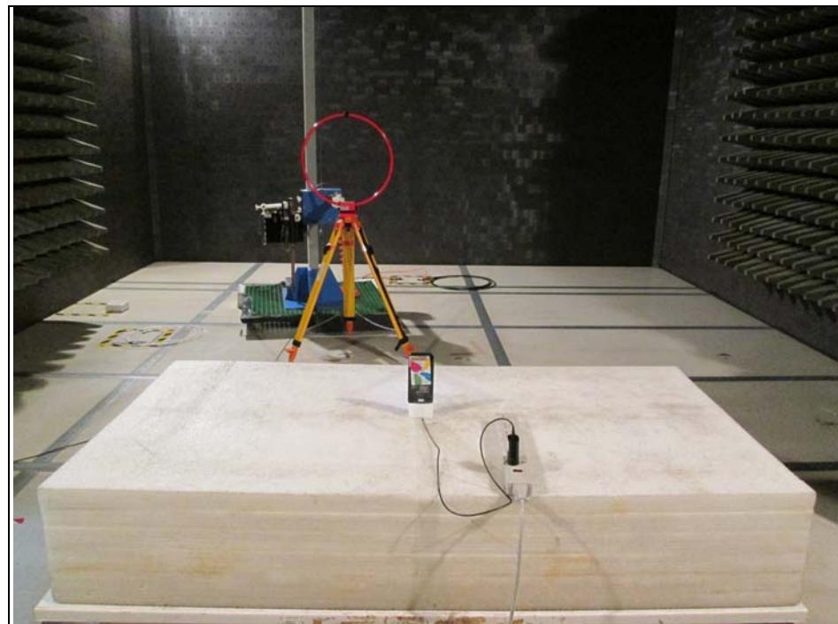
Radiated Emission Test (30MHz to 1GHz)
