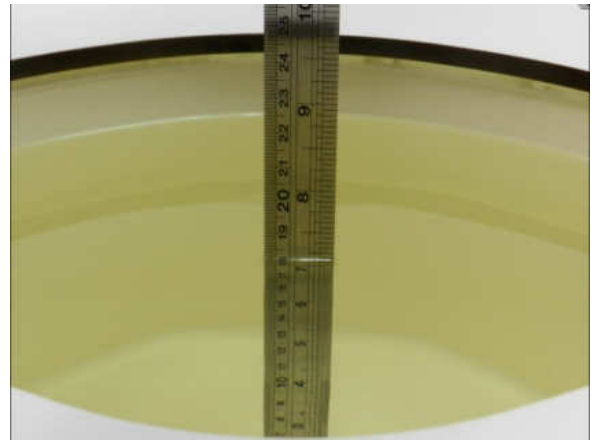
Fig 10.2 Photo of Liquid Height for Body SAR
