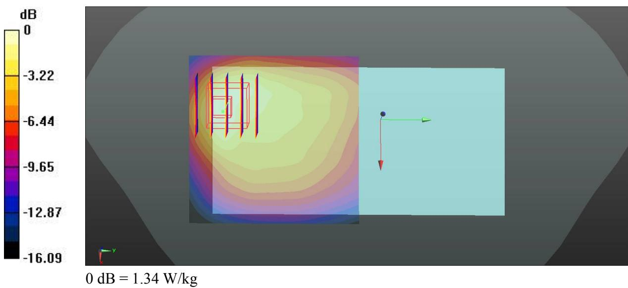
**36\_LTE Band 2\_20M\_QPSK\_1RB\_49offset\_Back\_10mm\_Ch18900**
