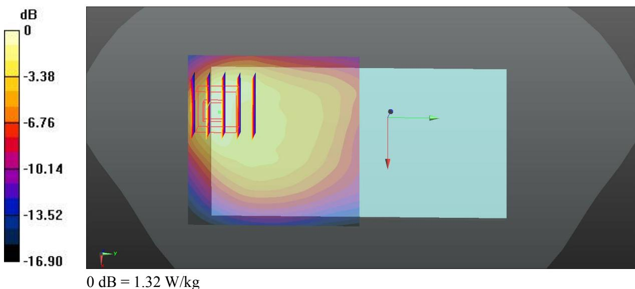
**32\_LTE Band 12\_10M\_QPSK\_1RB\_25offset\_Back\_10mm\_Ch23095**
