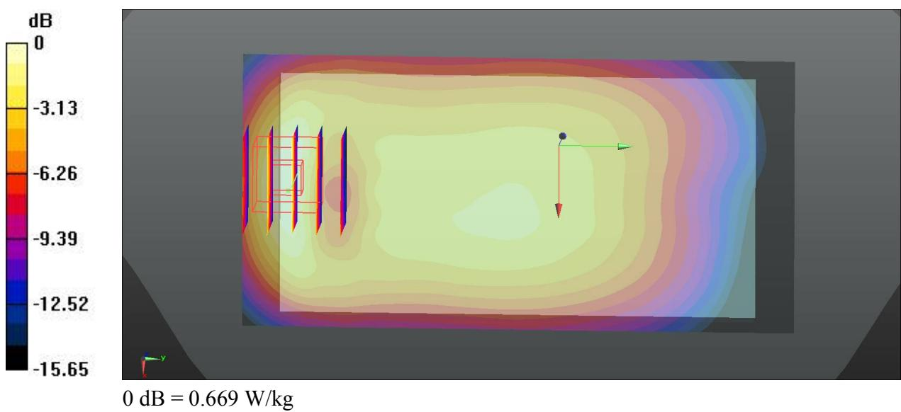
**35\_LTE Band 66\_20M\_QPSK\_1RB\_49offset\_Back\_10mm\_Ch132572**
