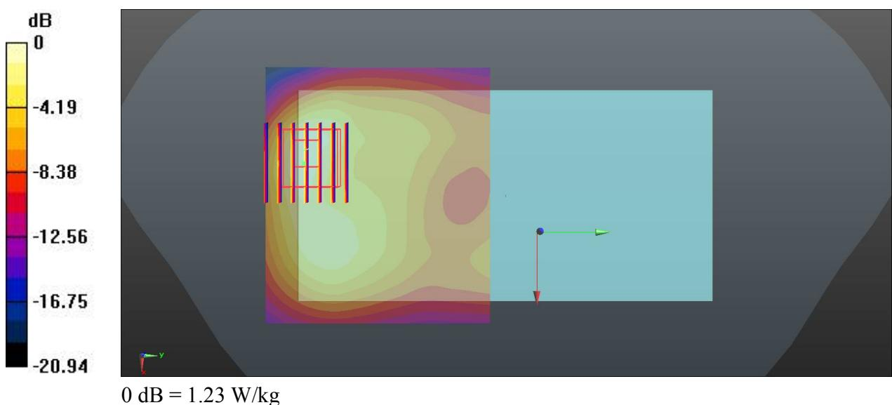
**38\_LTE Band 38\_20M\_QPSK\_1RB\_49offset\_Back\_10mm\_Ch38150**
