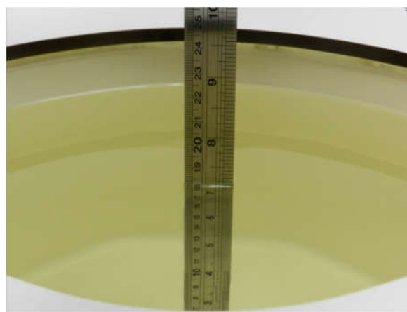
Fig 10.2 Photo of Liquid Height for Body SAR
