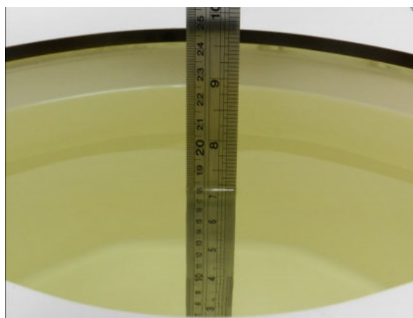
Fig 10.2 Photo of Liquid Height for Body SAR
