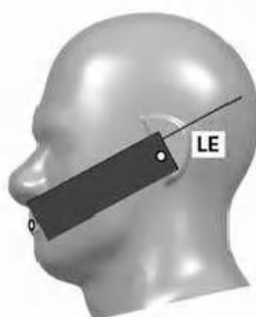
Fig 9.2.2 Handset vertical and horizontal reference lines—“clam-shell case”
