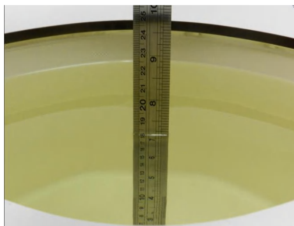
Fig 10.2 Photo of Liquid Height for Body SAR
