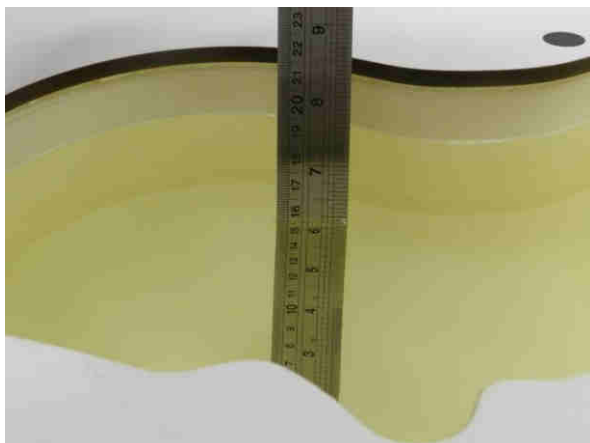
Fig 10.1 Photo of Liquid Height for Head SAR
