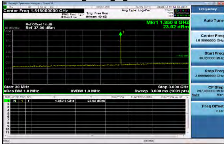
30MHz~3GHz HSDPA B2 LowCH9262-1852.4
