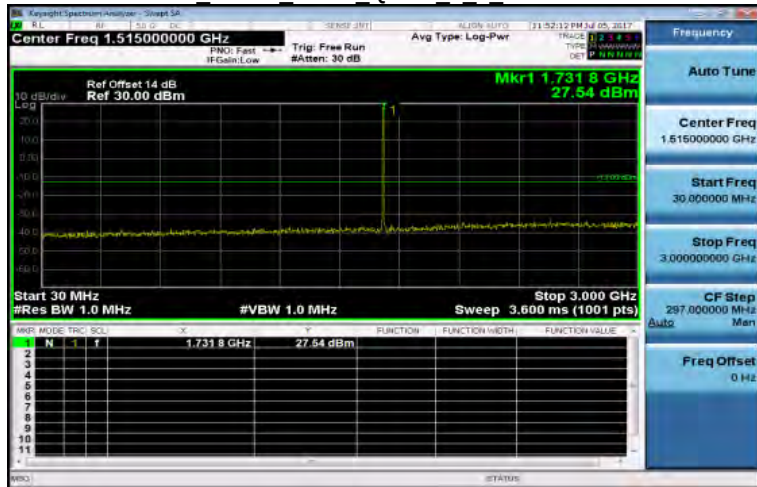
30MHz~3GHz Band4 3MHz QPSK 1 0 MidCH20175-1732.5
