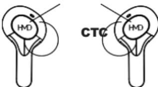
**Step 1:** To switch the earbuds on (Smart Power On), open the lid of the charging case when the earbuds are inside and the earbuds power on automatically. This is indicated by a solid LED light for few seconds .
