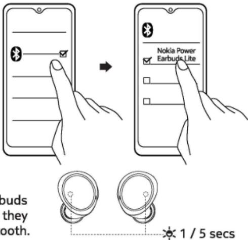
The LED indicator lights of the earbuds will flash blue every 5 seconds when they are successfully connected via Bluetooth.
