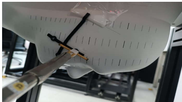
Dipole Placed at Location H in 90° Orientation (10mm Spacer)
