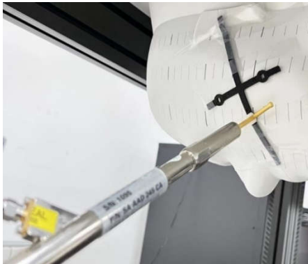
Dipole Placed at Location F in 90° Orientation (10mm Spacer)
