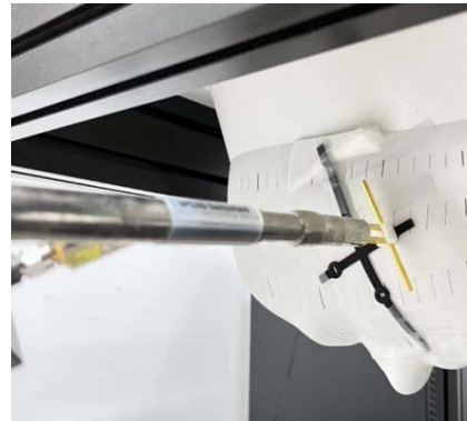
Dipole Placed at Location H in 0° Orientation (10mm Spacer)
