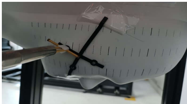
Dipole Placed at Location C in 90° Orientation (10mm Spacer)
