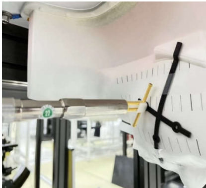
Dipole Placed at Location C in 0° Orientation (10mm Spacer)
