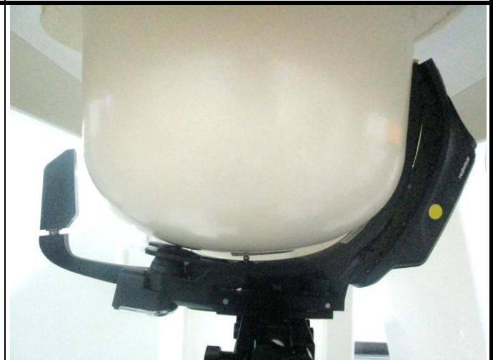
Test Position 8: Left Head (5G WLAN)
