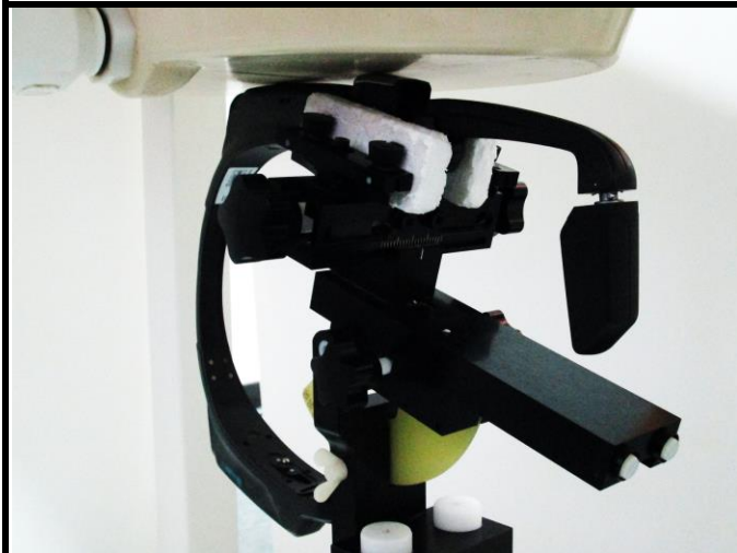
Test Position 11: Right Side (5G WLAN)
