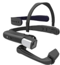
1. Position the HMT device such that main unit is positioned on the side of the head and the LCD pod is aligned in front of your left or right eye.
