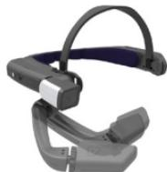
1. Move the LCD Pod forward or backward, to set the focus of the display screen. When set correctly the screen will be bright and crisp, and you can even read the smallest text.
