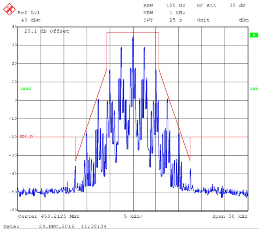
**Occupied Bandwidth –12.5kHz, 453.2125 MHz, Low Power Level**
