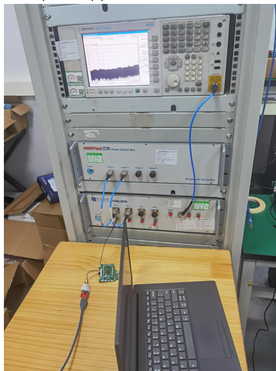
Test Setup Photo(s) of RF Conducted Measurement
