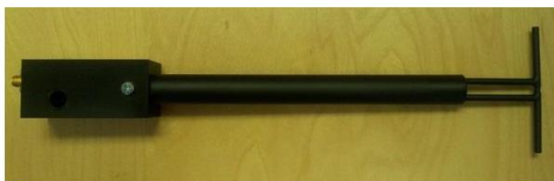
Figure 1 – MVG COMOSAR Validation Dipole
