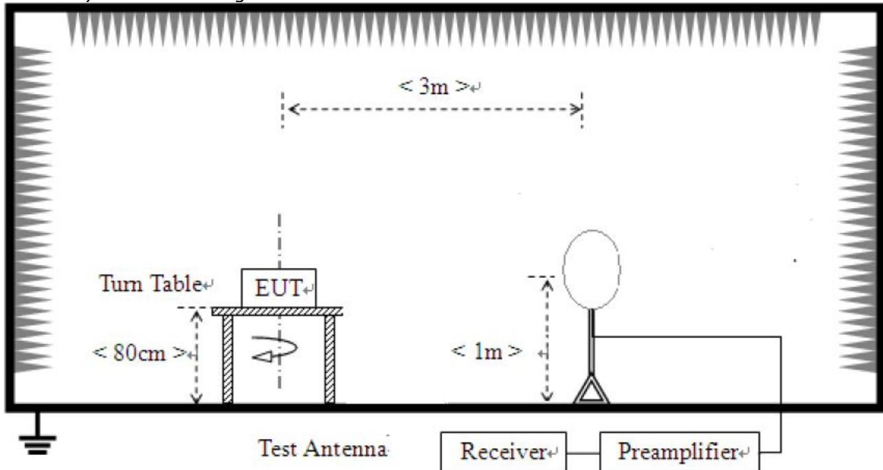
2) For field strength of emissions from 30 MHz to 1 GHz
