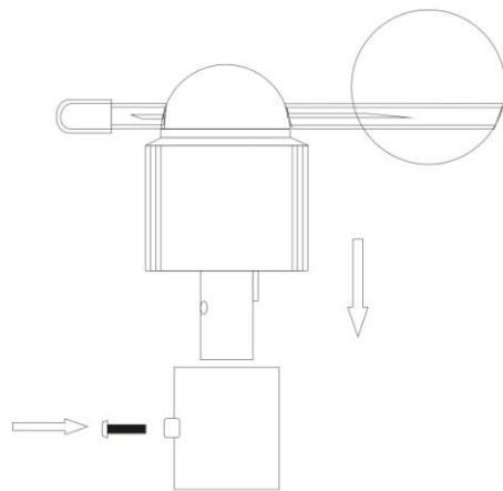
**Attention!!** Please align the “North” indicator sticker with the NORTH direction to enable it to record accurate reading
