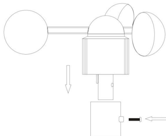
**3) Mounting the wind direction sensor to the ① bracket:** first check the wind direction sensor before fixing, the wind direction sensor should now be mounted onto the bracket provided to allow the wind to travel around the sensor unhindered from all directions. Then fix it with bolt and screw. there is one cable from wind speed sensor, please insert it into the socket under the wind direction sensor. please follow the below display:
