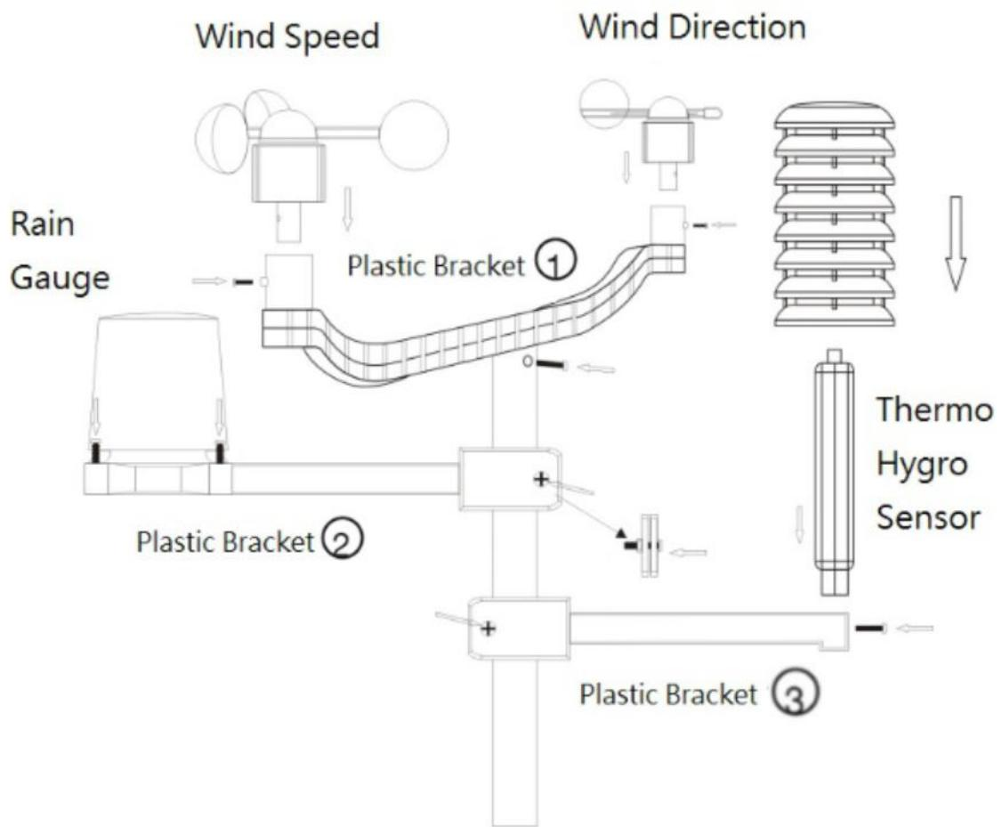
2) **Mounting the wind speed sensor to the ① plastic bracket:** first check the wind-fan can rotate freely before fixing. The wind speed sensor should now be mounted onto the bracket provided to allow the wind to travel around the sensor unhindered from all directions. Then fix it with bolt and screw. Please follow the below display:
