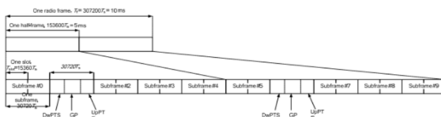
Figure 4.2-1: Frame structure type 2 (for 5 ms switch-point periodicity)
