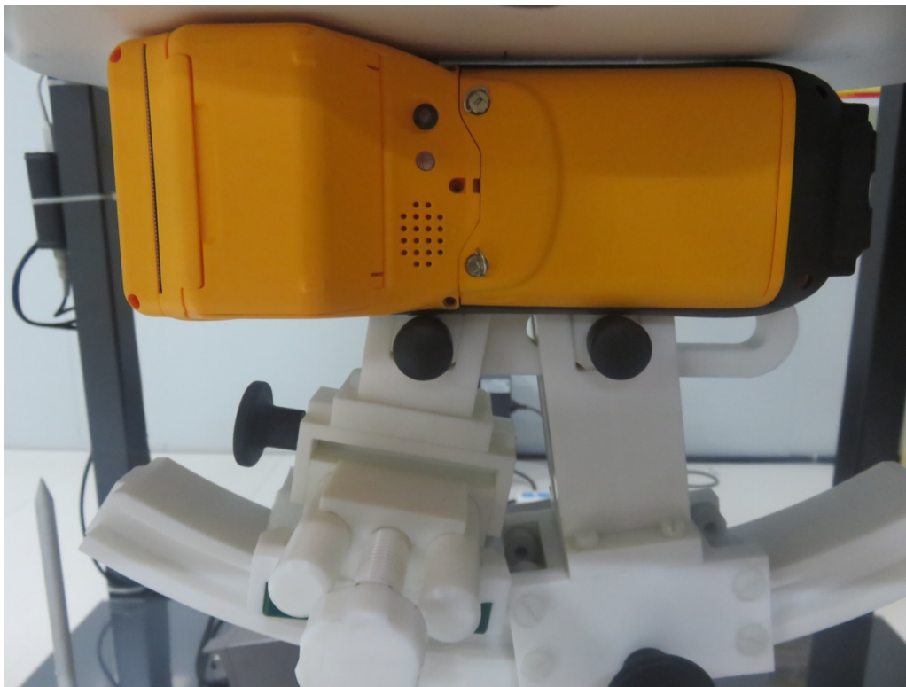
0mm body-worn Left Side Setup Photo(hotspot)
