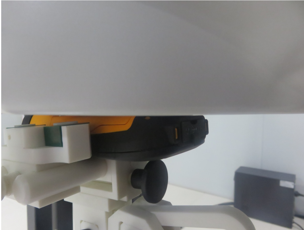
0mm body-worn Back Side Setup Photo(hotspot)
