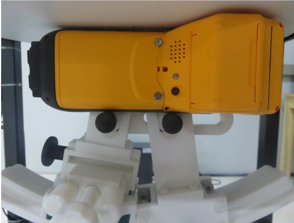
0mm body-worn Right Side Setup Photo(hotspot)
