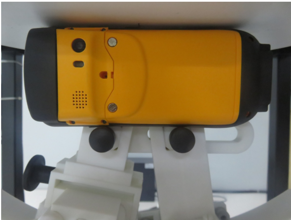
0mm body-worn Left Side Setup Photo(hotspot)
