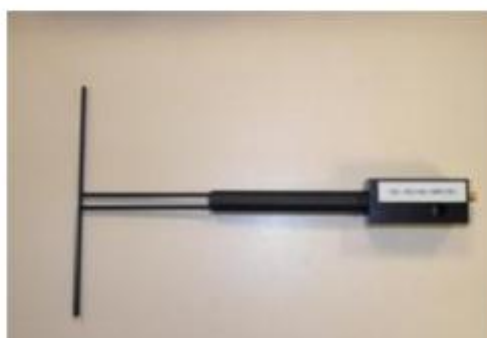
Figure 1 – Satimo COMOSAR Validation Dipole
