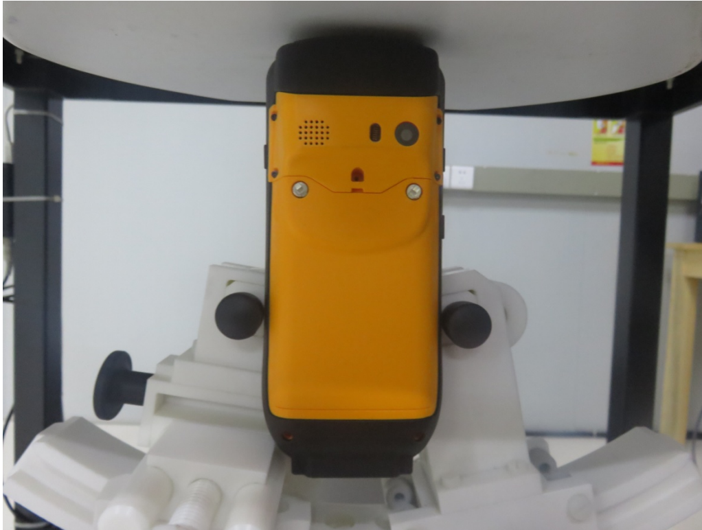
0mm body-worn Top Side Setup Photo(hotspot)
