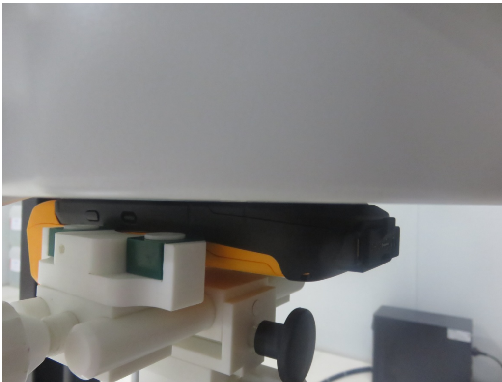
0mm body-worn Front Side Setup Photo(hotspot)
