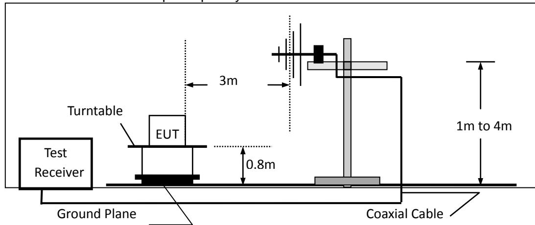
(C) Radiated Emission Test-Up Frequency Above 1GHz
