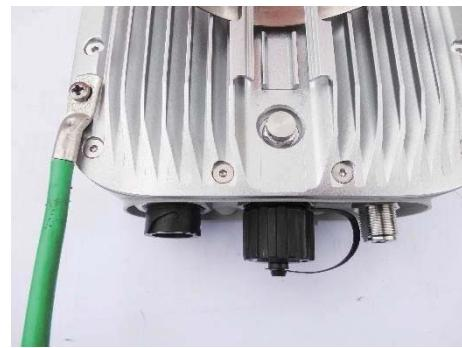
**IMPORTANT:** It is not permitted to ground the gateway directly to the tower structures.
