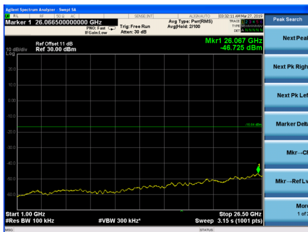
GFSK on channel 01
