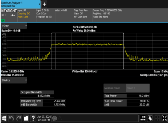
B2_N48(5M)_CP-OFDM_256 QAM Outer Full Mid CH
