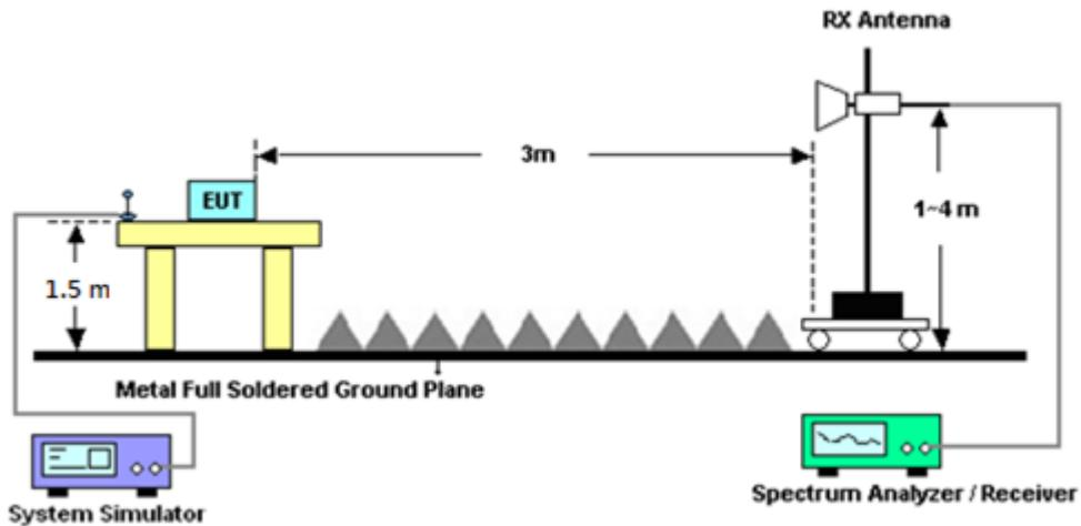
For radiated test above 18GHz
