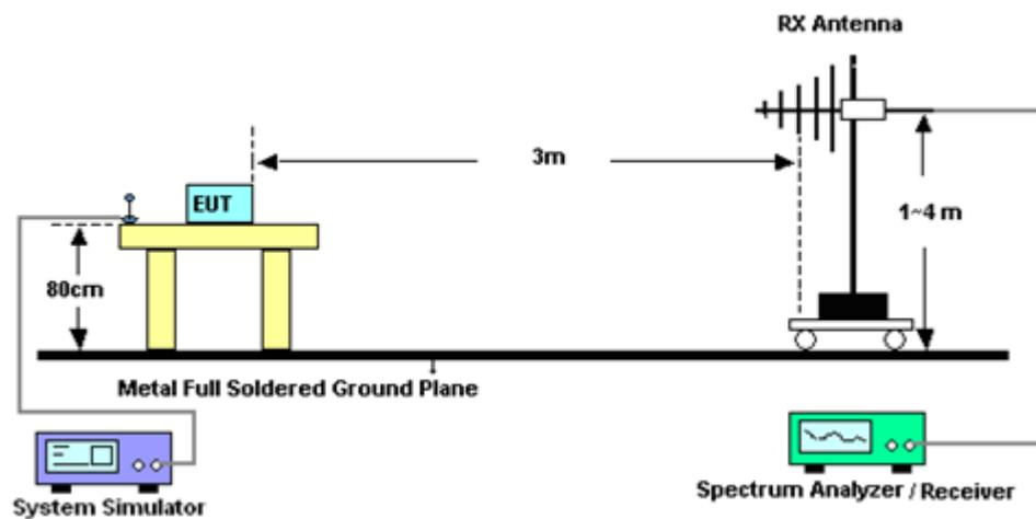
For radiated test above 1GHz
