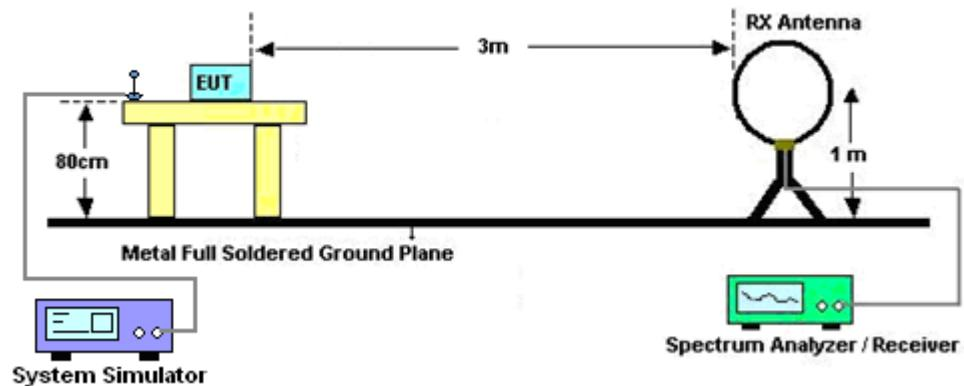
For radiated test from 30MHz to 1GHz
