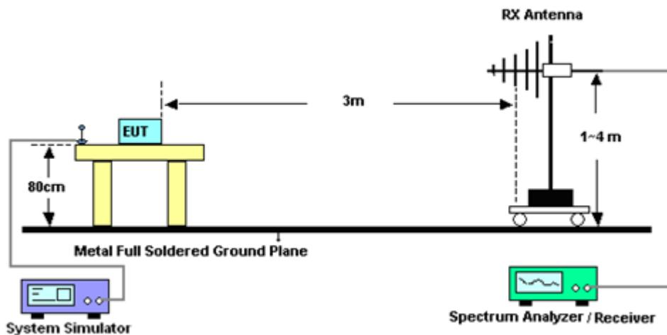
For radiated emissions from 1GHz to 18GHz
