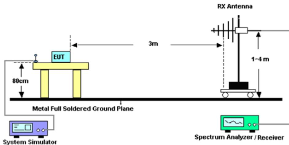
For radiated emissions from 1GHz to 18GHz
