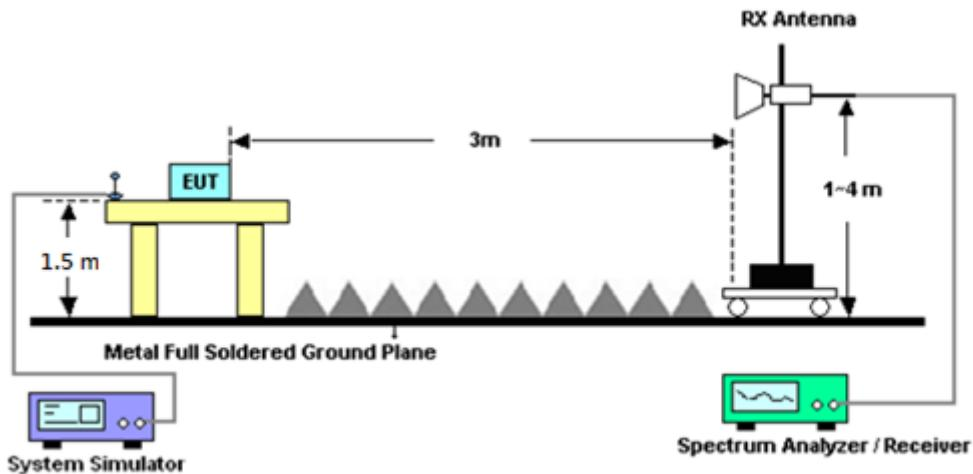
For radiated test above 18GHz
