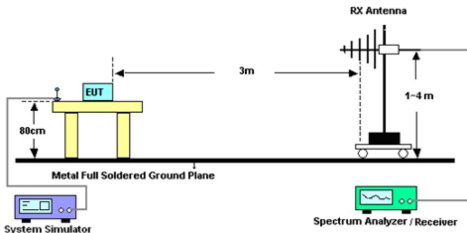
For radiated emissions from 1GHz to 18GHz
