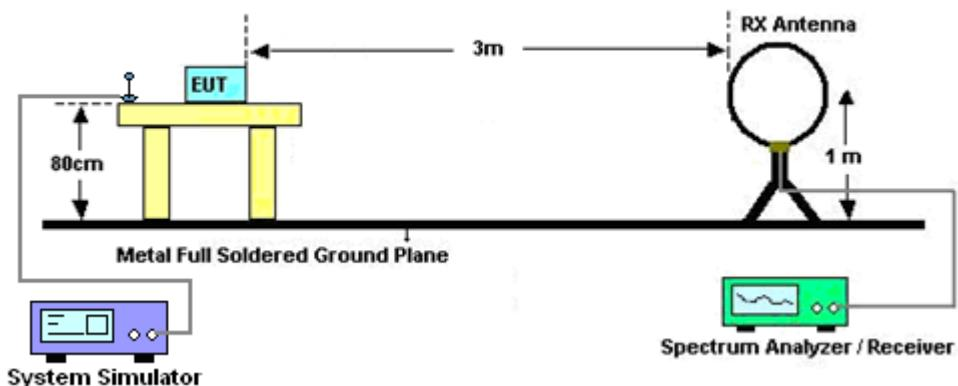
For radiated test from 30MHz to 1GHz
