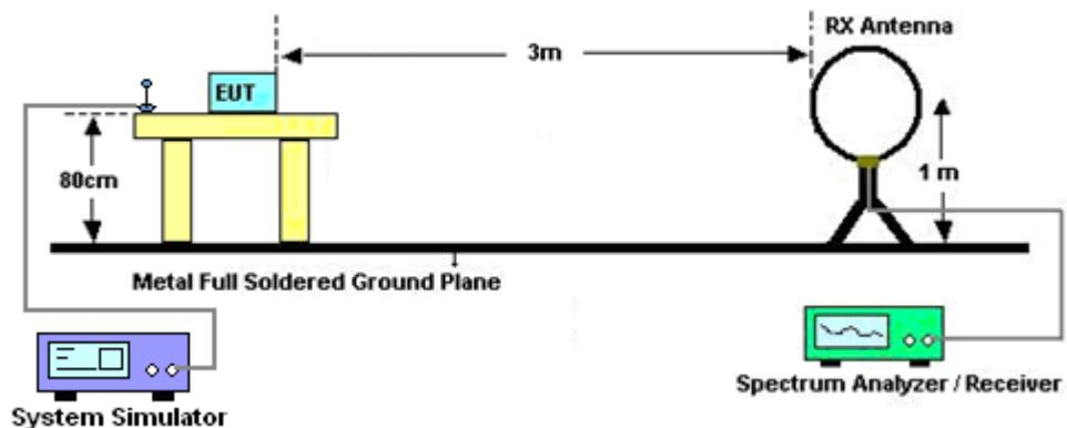
For radiated test from 30MHz to 1GHz
