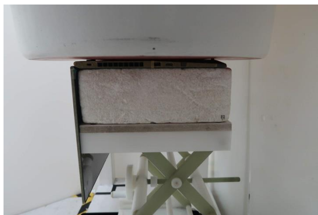
Bottom of Laptop, Test Separation 0 mm
