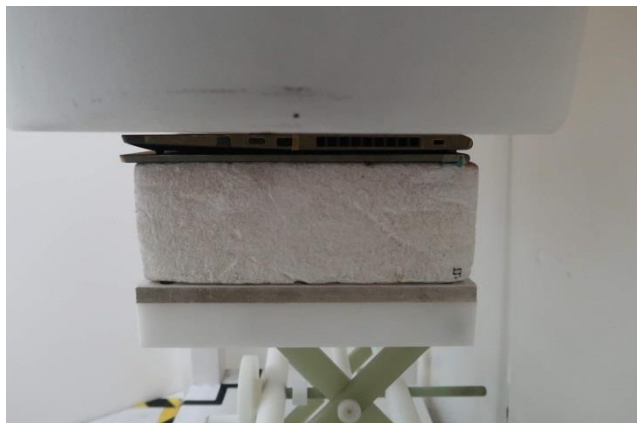
Bottom Face, Test Separation 0 mm
