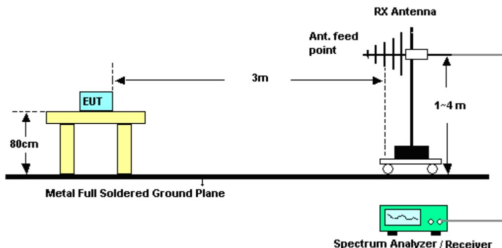
**For radiated emissions above 1GHz**
