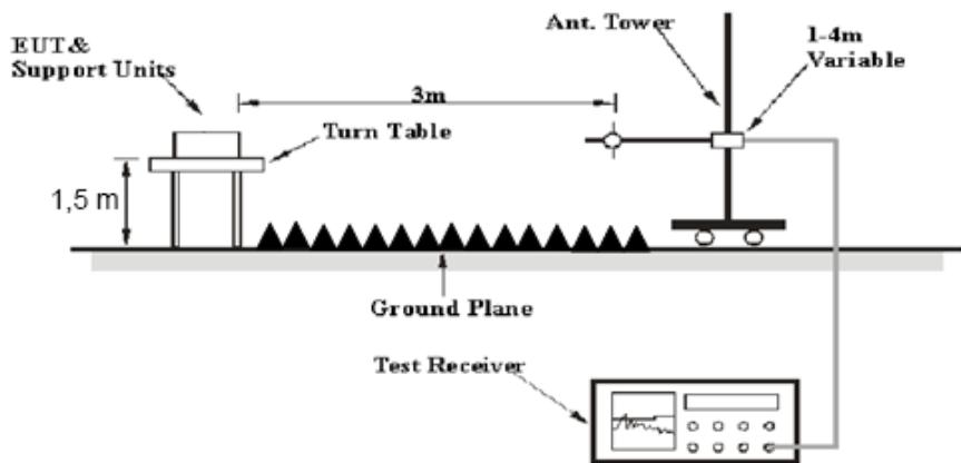
The radiated emission below 1GHz tests were performed in the 10 meters chamber test site, above 1GHz tests were performed in the 3 meters chamber test site A, using the setup accordance with the ANSI C63.10-2013. The specification used was the FCC 15.209, and FCC 15.247 and the RSS-247 Clause 5.5, RSS-GEN Clause 8.10 limits.
