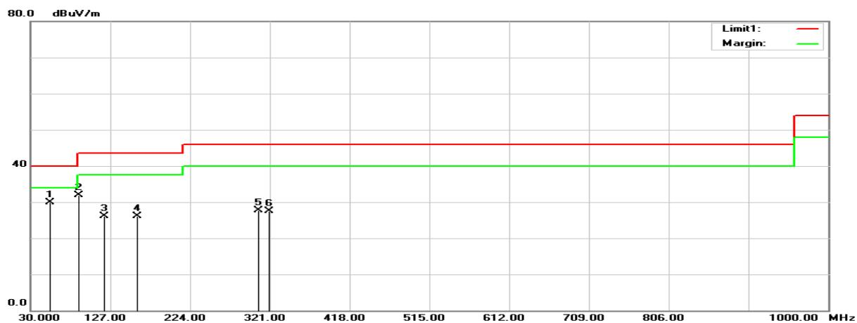
**Pygate, DC 48V from PoE****30MHz-1GHz:****Horizontal**
