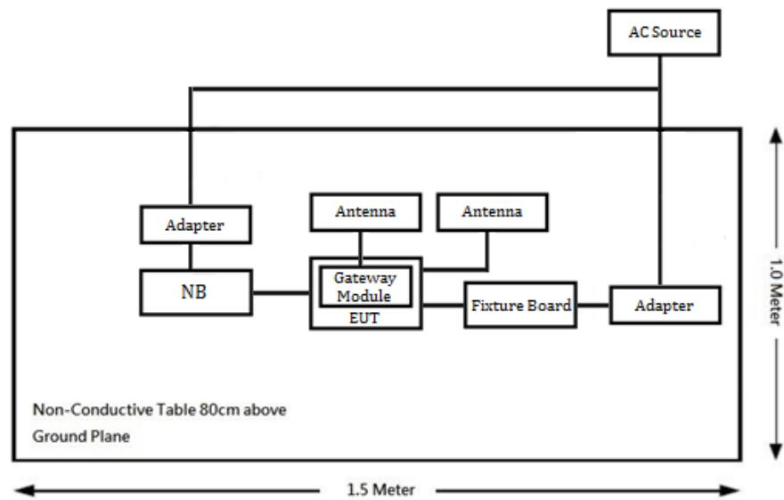
Pygate, DC 5V from USB Port + Gateway Module (GPy 1.0)
