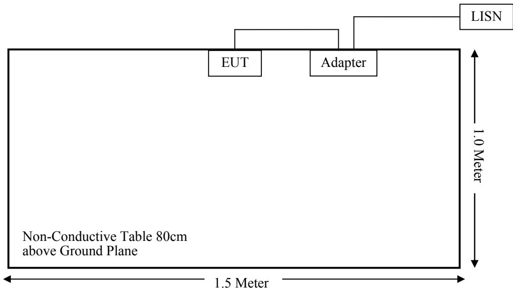
For Radiated Emissions(Below &amp; Above 30MHz):
