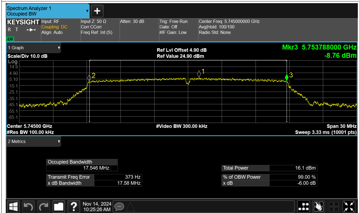
-6dB Bandwidth NVNT ac20 5785MHz Ant1
